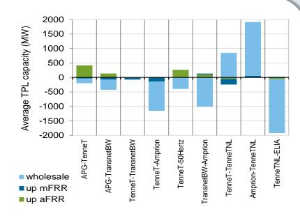
For the transmission line APG-TenneT positive values mean, that APG provides upward FRR or exports energy to TenneT, negative vice versa.
